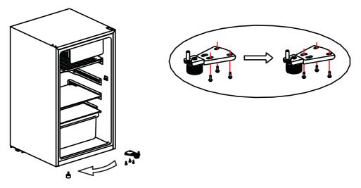
**Step 4** Put the door on the bottom hinge and assemble the upper hinge, upper hinge cover and plastic screw hole caps successively.
